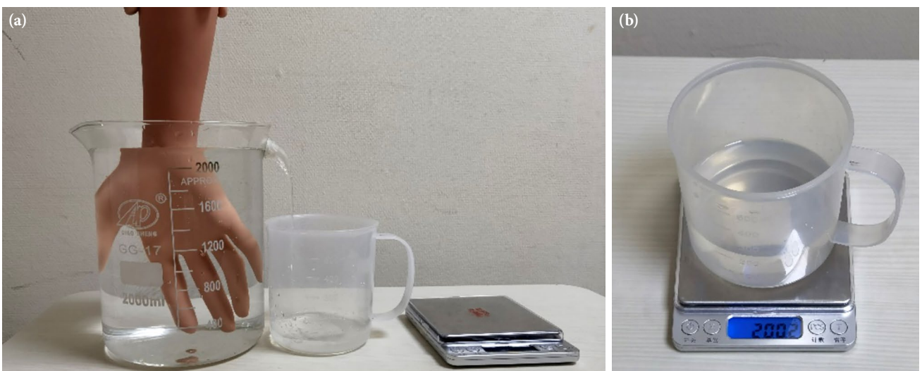
Figure 2. (a) An assistant helped the subject hold the hand perpendicular to the surface of the water and immerse it in the water, and the water overflowed into the measurement cup. (b) When the water stopped overflowing, the mass of the spilled water was weighed to calculate the volume of the hand.
