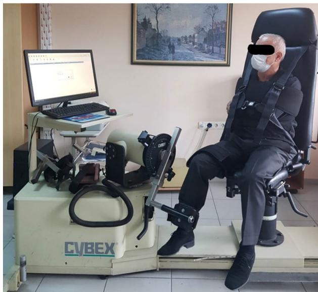
**Figure 2.** A stroke survivor performing the isokinetic strength test of the non-paretic knee.
