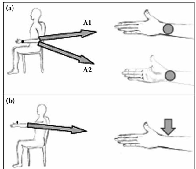
**Figure 2.** Strength test. (a) A1: Participant positioned on a chair for external rotation strength test (A1) and internal rotation (A2) (A1 and A2: circles indicate the arm location where perpendicular force was applied). (b) Participant positioned on a chair for scapular plane abduction strength test (b: vertical arrow indicates the direction of applied force)
