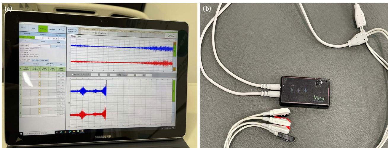
**Figure 2.** The surface electromyography (sEMG) (a) User interface of sEMG software (MoTive-Rs, version 1.0). (b) Bluetooth sEMG device (MOT10).
